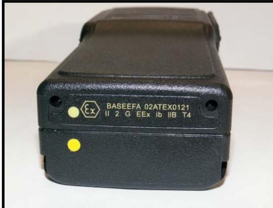
Fig 3. ATEX Radio & Battery correctly installed
