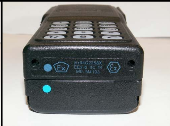
Fig 4. Cenelec Radio & Battery correctly installed
